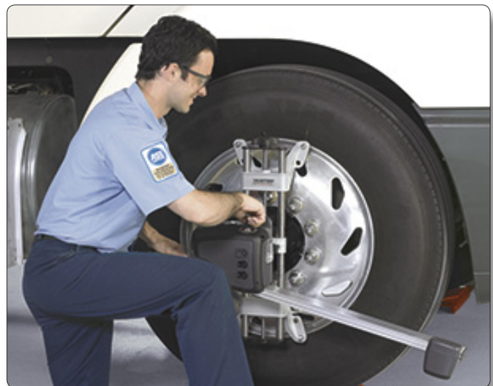
Optional cordless sensors are faster to set up and easier to use.
